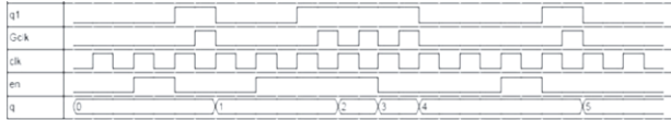
Figure 19 Normal output of negative edge counter when positive latch based OR Gated Clock is used
