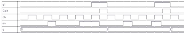
Figure 20 Output of negative edge counter when there are some random hazards at En
