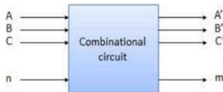
Figure 1 Block diagram of combinational circuit
